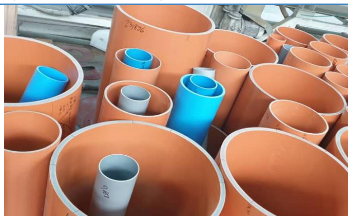
Figure 11: PVC pipes (orange ones are for residual water)
